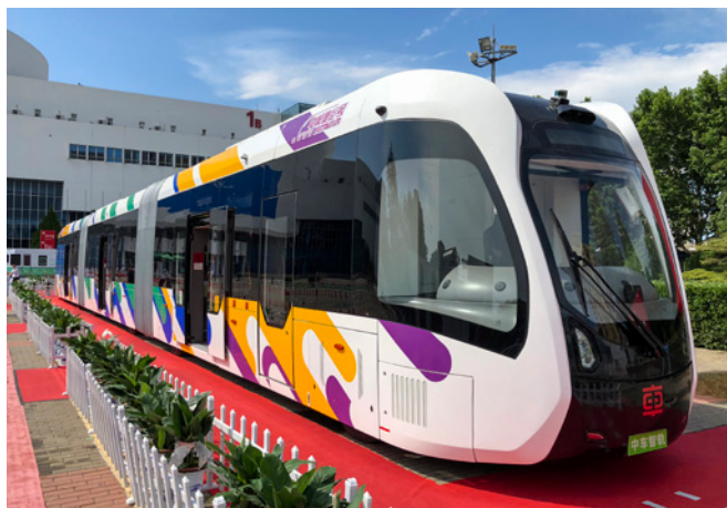
Autonomous-rail Rapid Transit train, already in experimental operation in Zhuzhou.
